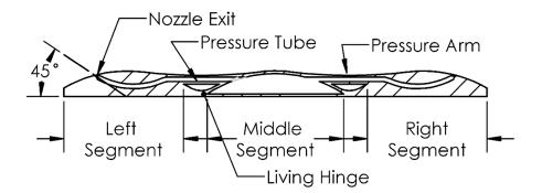
Figure 4: A cross-section of the spray compliant device exposing the device's interior components, the location of the pressure arm, and the angle of nozzle sprout.
