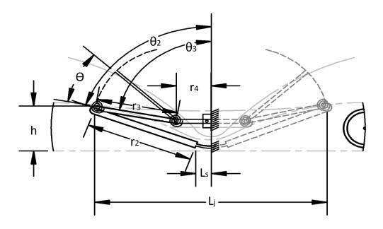
Figure 9: The fully compliant device in which the configuration shows a slider system. The middle of the fully compliant device is considered the base on which the slider vertically slides.
