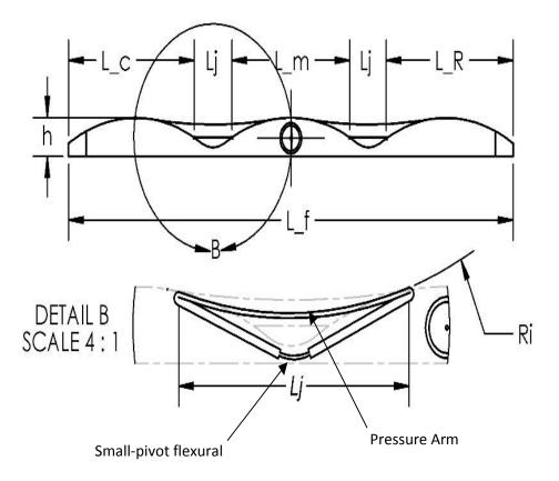
Figure 8: A magnification of the left and middle sections. Illustration B shows the joint skeleton of the device.
