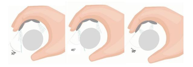
Figure 5: Angle of the nozzle from the base of the spray device. The angle lies at  $30^{\circ}$ ,  $45^{\circ}$ , and  $90^{\circ}$  to show the total coverage when an object is gripped.
