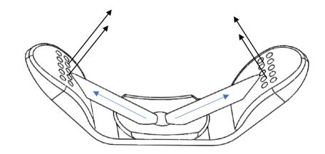
Figure 6: Deformed configuration of the compliant spray device with spout out direction.
